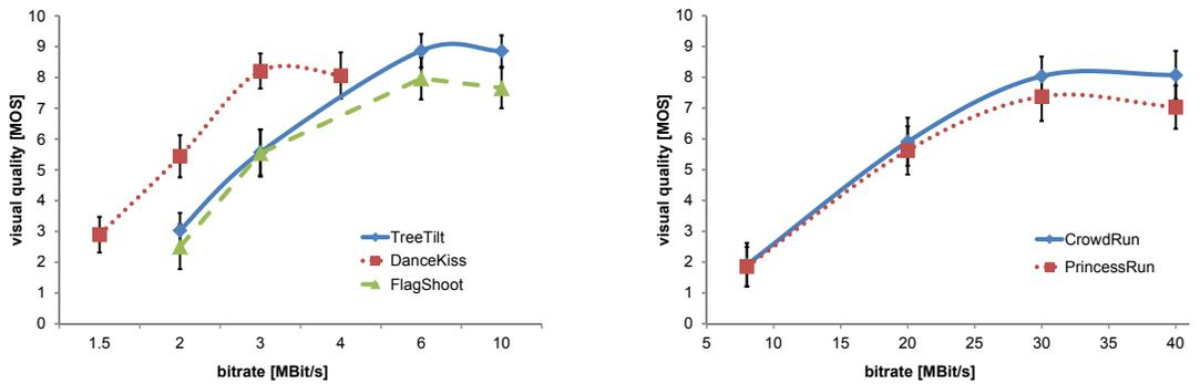
Fig. 9: 1080p50 dataset: visual quality at bitrates from 1.5 Mbit/s to 40 Mbit/s with the reference display for different video sequences. The whiskers represent the 95% confidence intervals of the subjective test results for the visual quality
